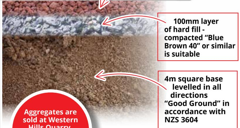
100mm layer of hard fill - compacted "Blue Brown 40" or similar is suitable
