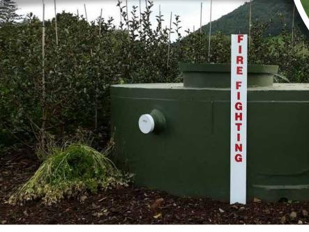
The Duracrete 9,000 Litre tank is the smallest model of Duracrete tank at 9000L capacity. Often used as a header tank on properties. This can be placed above ground or partially buried to 1.65m maximum.The tank is 2.5m diameter.
